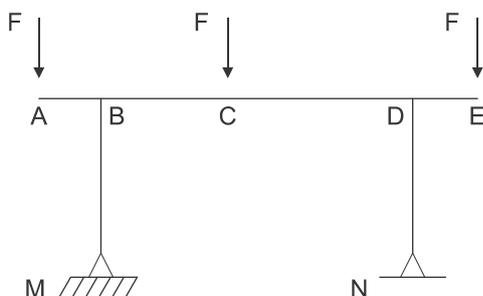
Dados:  $F = 10 \text{ kN}$ ;  $AB = DE = 2 \text{ m}$ ;  $BC = 4 \text{ m}$ ;  $CD = 6 \text{ m}$  e  $BM = DN = 5 \text{ m}$
